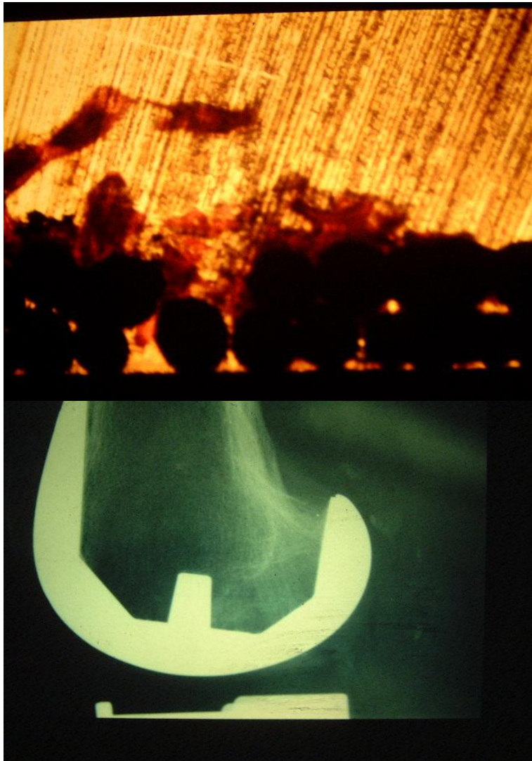
Figure 13: Top picture is an electromicrograph showing incorporation of bone (red) onto the surface of the hydroxyapatite. Bottom picture shows an x-ray of an uncemented, hydroxyapatite coated total knee replacement. There are no gaps in the bone-prosthesis junction indicating incorporation of the bone onto the prosthesis.
